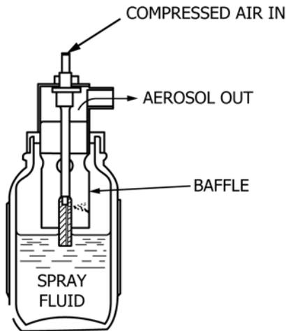
FIG. 3 Collision Atomizer
