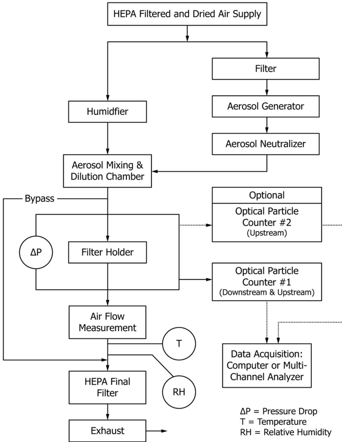
FIG. 1 Schematic of Test Method
