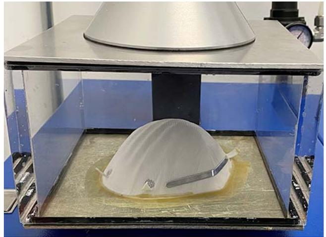
FIG. 1 Example of a Filter Holder Adapter
